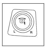
The outside power mirror control is located on the driver side door.
